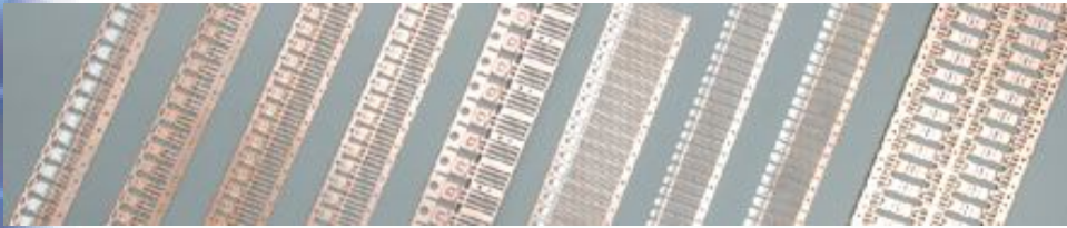
Lead Frame of Semiconductors for Discrete Devices
