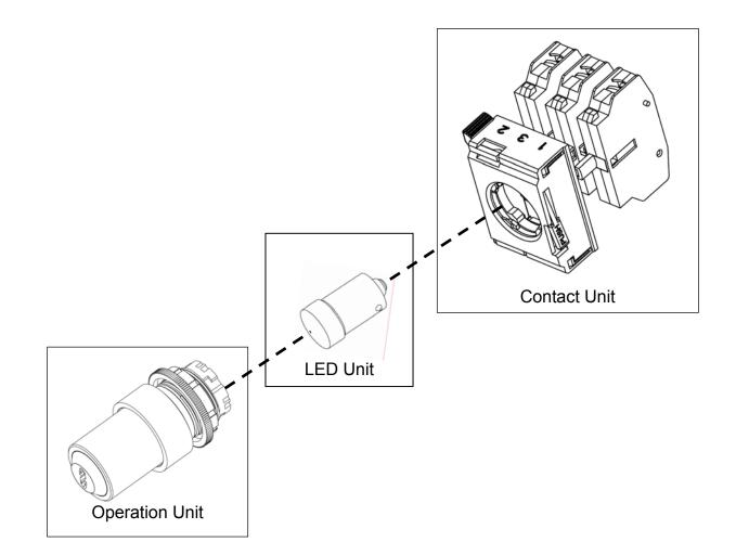
Operation unit, LED unit, and contact unit (contact blocks) can be sold separately. Please see [4.Part numbering system] for operation unit part number. For other accessories (LED lamp, contact block, etc.), please refer to accessory part in catalog.
