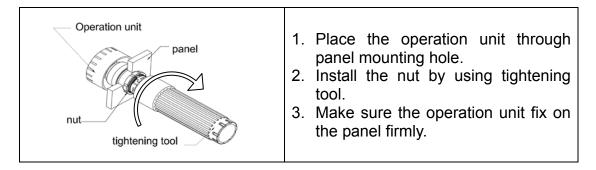
5-3. Operation unit and contact unit installation
