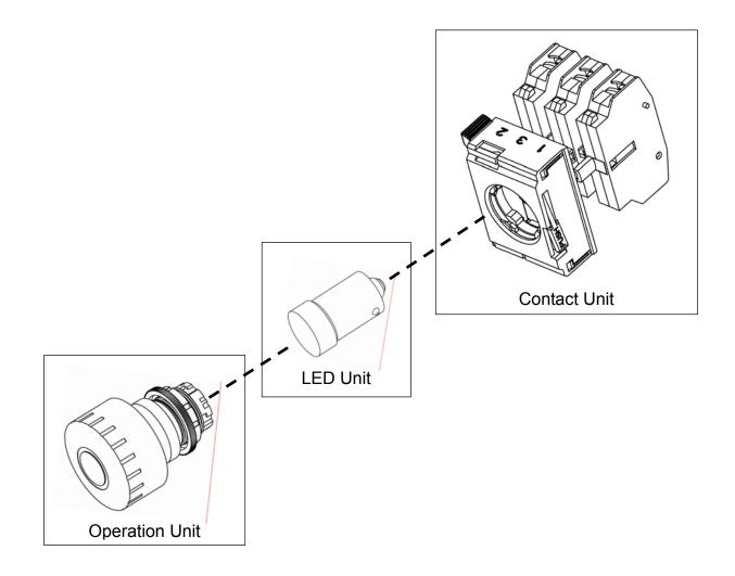
Operation unit, LED unit, and contact unit (contact blocks) can be sold separately. Please see [4.Part numbering system] for operation unit part number. For other accessories (LED lamp, contact block, etc.), please refer to accessory part in catalog.
