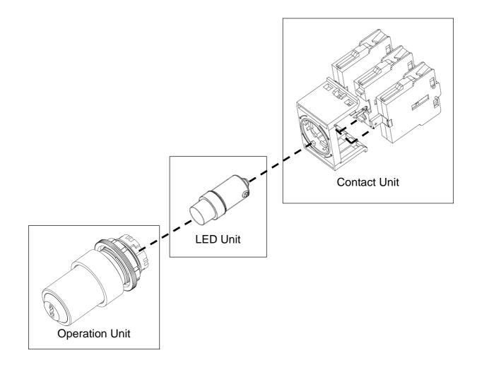
Operation unit, LED unit, and contact unit (contact blocks) can be sold separately.
